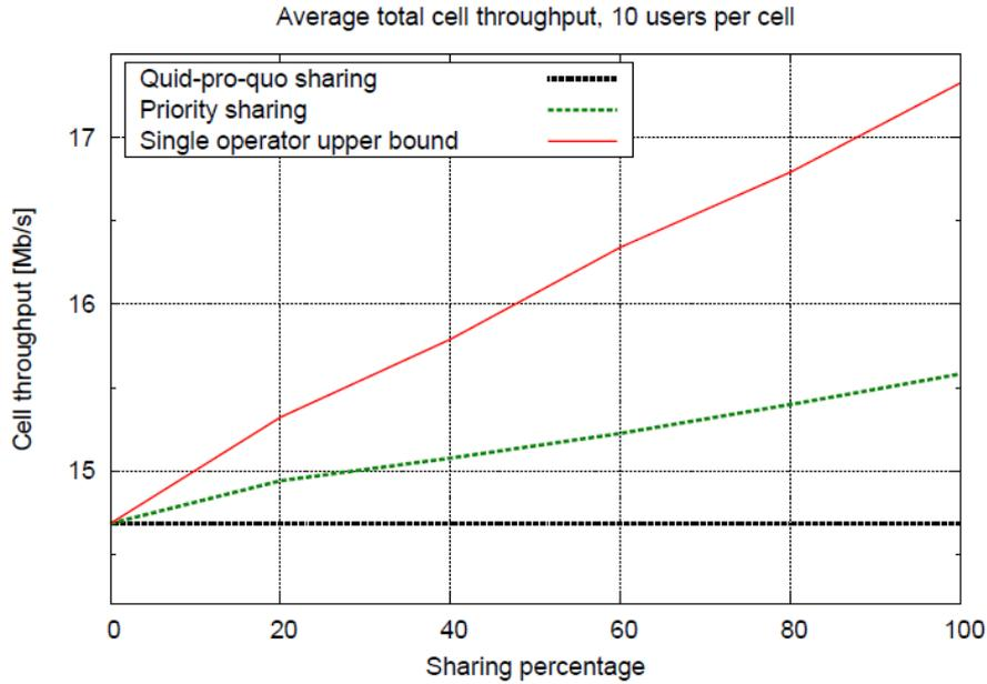
**Figure 2. Cell throughput as a function of the sharing percentage, maximal throughput scheduling**
