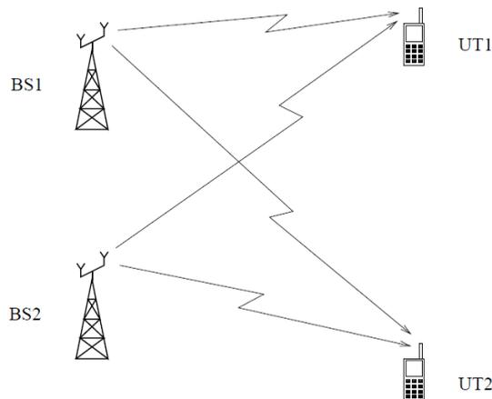
**Figure 3. Two-user MISO interference channel**
