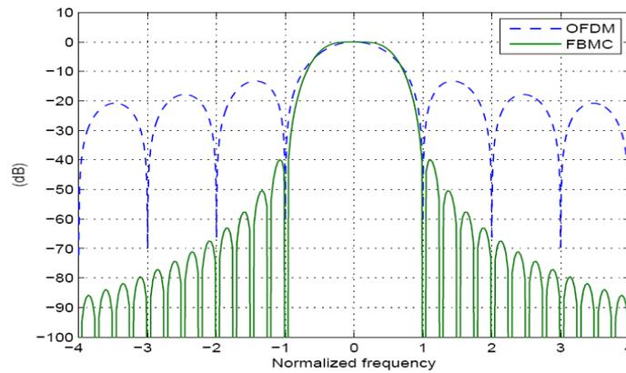
**Figure 6: Subcarrier PSD's of the OFDM and FBMC systems.**
